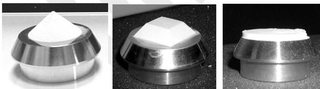
Figure 3.6 – Photographs of pile shapes studied: Cone H, d, Obelisk and Wafer
