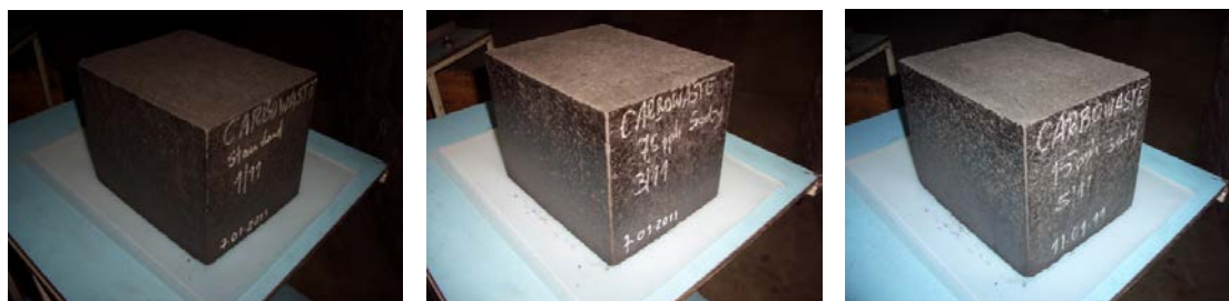
Figure 5.2 - Samples after block-pressing (from left to right: Reference, Trial 1 with 7.5 % carbon black, Trial 2 with 15 % of carbon black)
