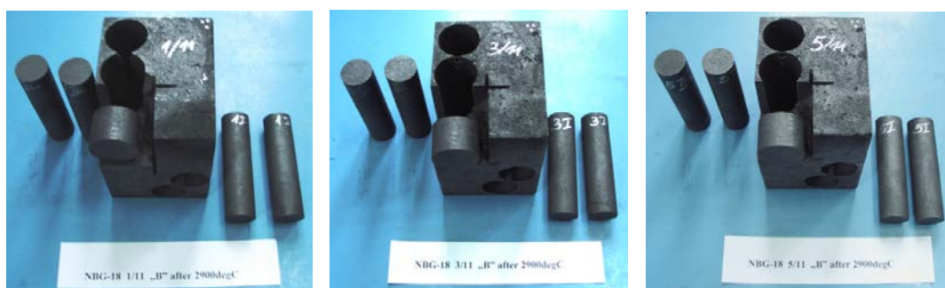
Figure 5.3 - Samples after graphitization (from left to right: Reference, Trial 1 with 7.5 % carbon black, Trial 2 with 15 % of carbon black), with core samples already taken
