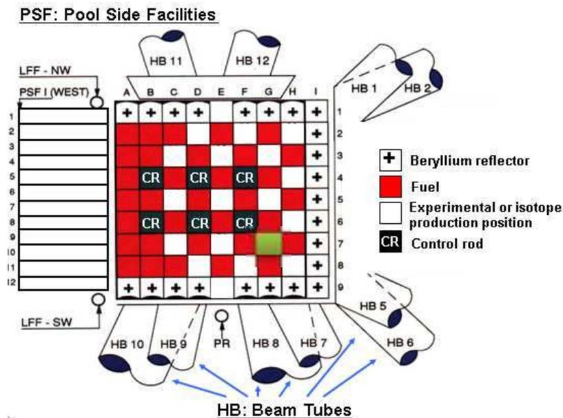
Figure 4-4 : Schematic view of the HFR core with the proposed irradiation position in green
