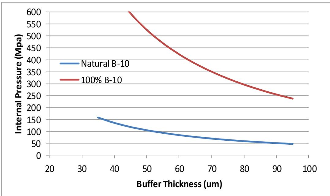
Figure 3. Nominal particle after 250 effective full power days of irradiation.
