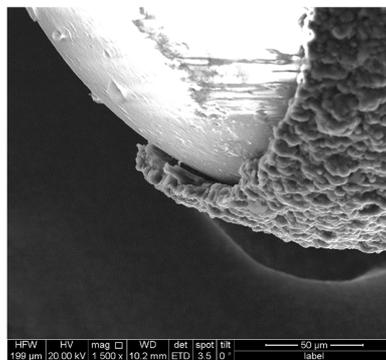
Figure 3-4 : SEM image of the deposit of supposed B<sub>4</sub>C
