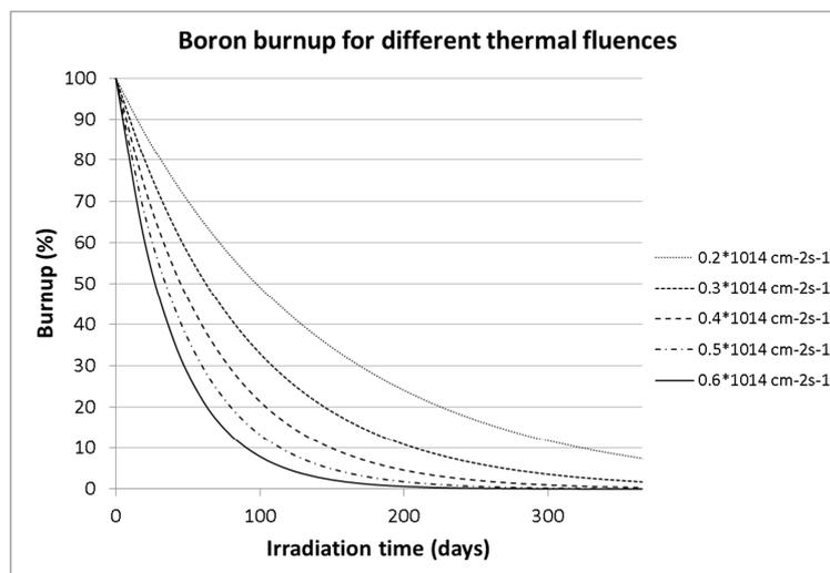
Figure 2-1: Estimated  $^{10}\text{B}$  burnup times for different fluences
