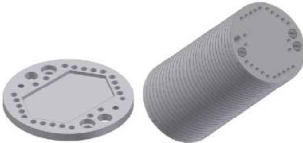
Figure 4-1 : Disc with hexagonal shape on the left, and a stack of discs on the right.
