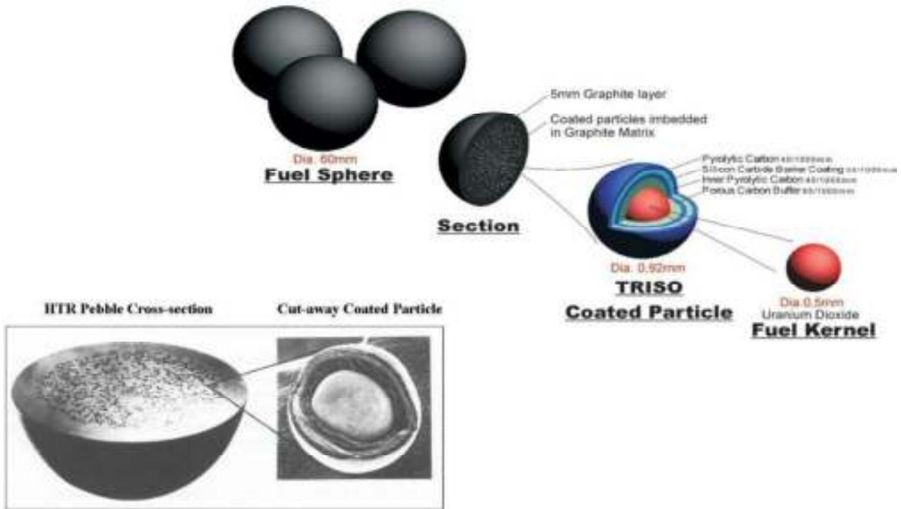
Figure 1 TRISO particles in HTR fuel technology
