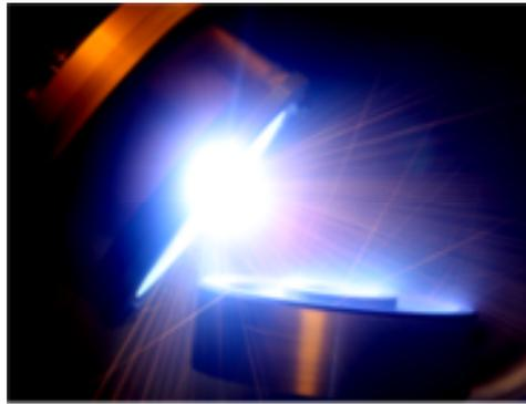
Figure 3-2 : Deposition of the Boron Carbide on the target (spraying observed due to the low density of the target)
