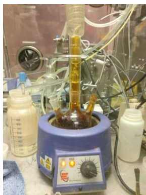
Fig.7: nitric distillation for concentration and denitration of a Pu solution
