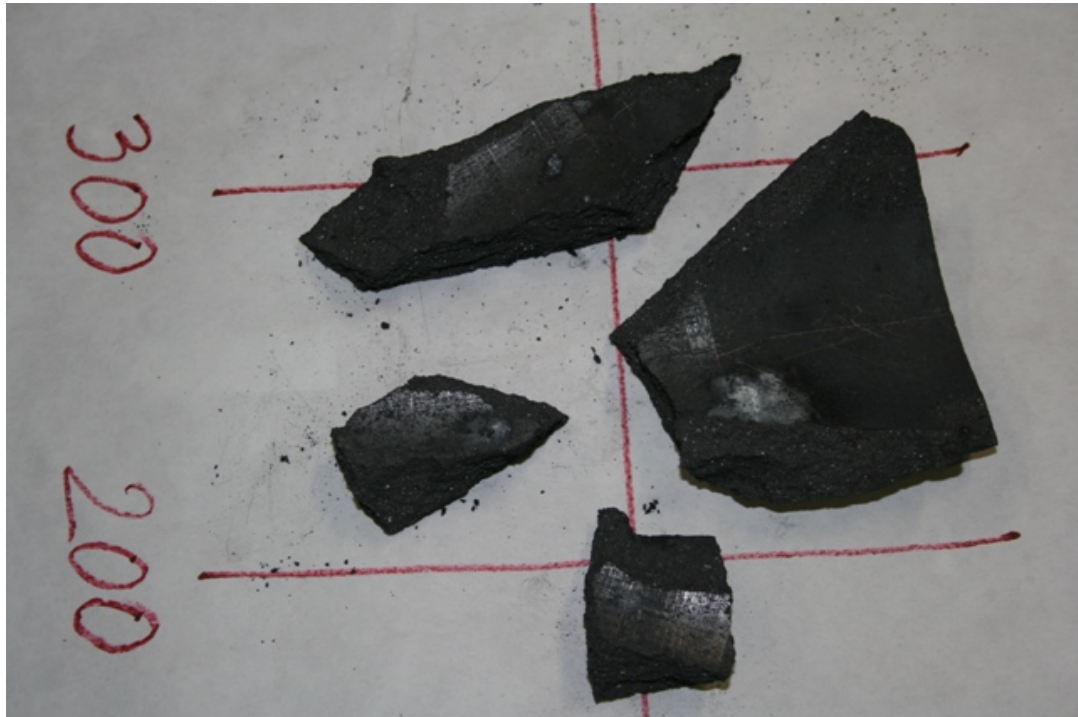
Fig. 13. The biggest (146g) sample (Gr.16) of irradiated graphite taken from the bottom part of the fuel assembly
