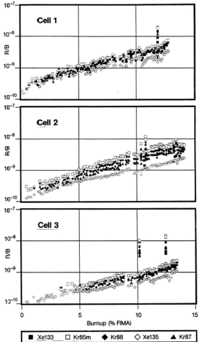
Fission gas release as a function of burnup in FRJ2-K15. R/B spikes visible during the +150°C temperature transients still do not reach the level of failure on one particle which would be at R/B around  $1 \times 10^{-6}$ .
