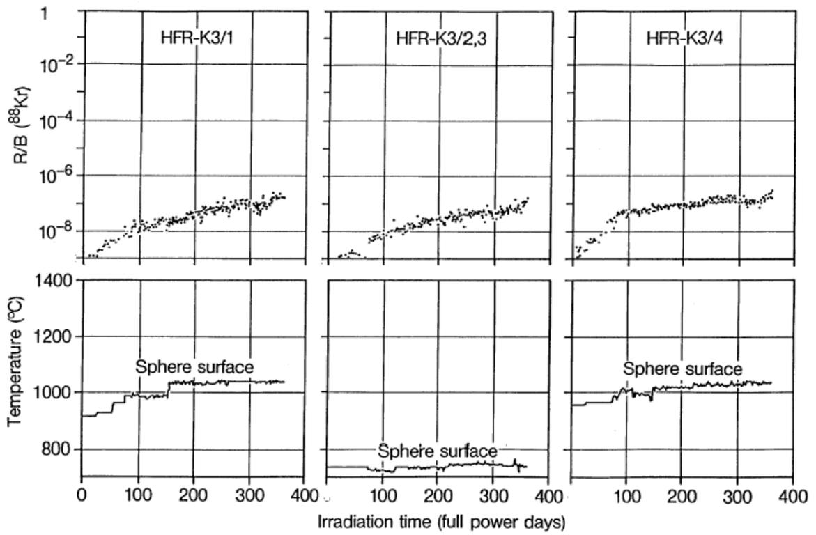
Fission gas release and surface temperatures of spherical fuel elements in HFR-K3
