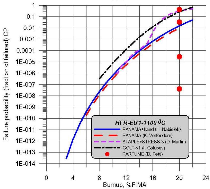
Prediction of coated particle failure probability for HFR-EU1 irradiation test with different computer models
