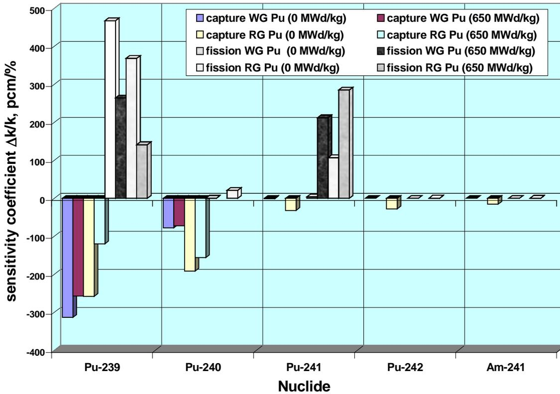
**Fig. 1: Comparison of sensitivity coefficients for capture and fission for RG and WG plutonium for 0 and 650 MWd/kg HM burnup**
