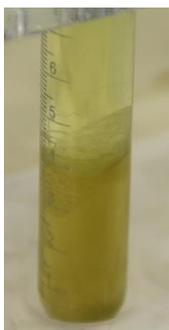
Some issues were experienced during the large scale batch tests: after the first step, third phase formation was observed at the interface between the organic and aqueous phases. The third phase was removed from the vial before the experiments were continued as planned. These results established the need for investigating third phase inhibitors in the next term.
