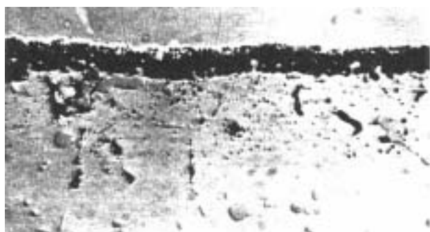
INLET SPECIMEN: decarburised -0.028 %C
