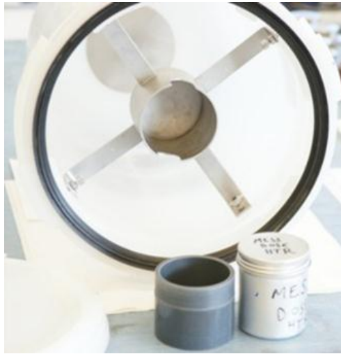
Fig. 4: La Calhene docking system for high activity cold plate samples
