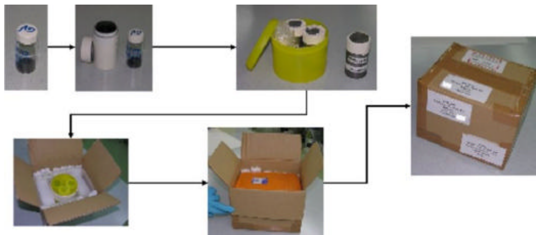
Figure 4.8 Conditioning samples to transport
