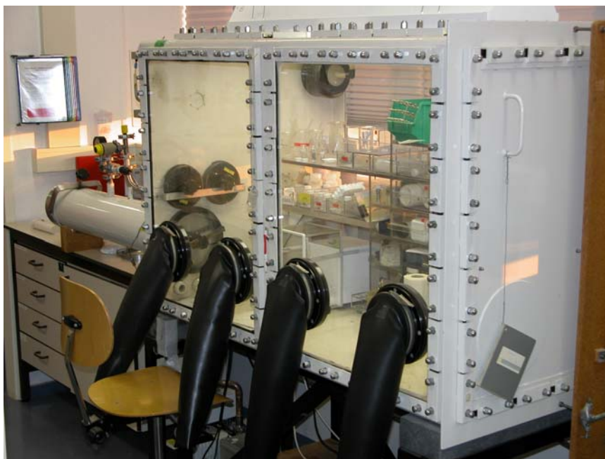
Figure 8: Argon-filled glove box for corrosion studies under inert atmosphere
