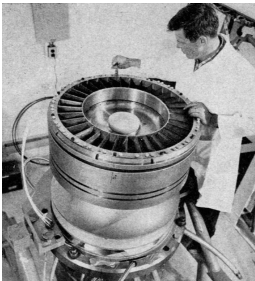
Fig. 3.17: Helium circulators of Fort St. Vrain a) view of the axial flow compressor b) view of the whole component
