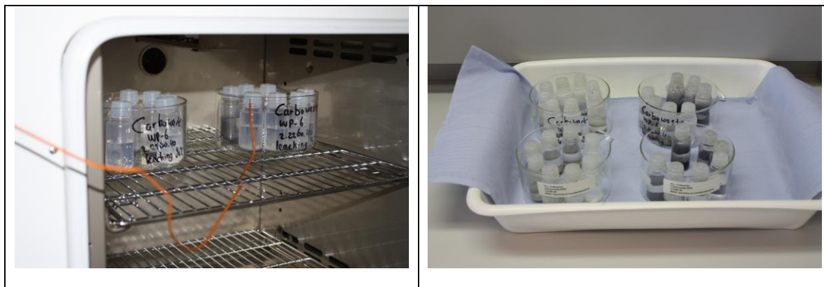
Figure 2-1 Picture of the leaching experiments – left at temperature of 90°C (controlled by certified probe) and right – at room temperature
