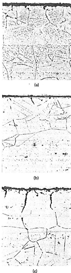
Fig. 16: Oxidation of Alloy 800H1 in V/HTR helium and in air at 750 °C: a) Specimen annealed in vacuum before exposure in helium (10 000 hours) without stress performed thick oxide scale and precipitation of carbides, b) specimen not annealed before exposure (10 000 hours, stress), c) specimen annealed in vacuum, tested in air (12 000 hours, strain) [23]
