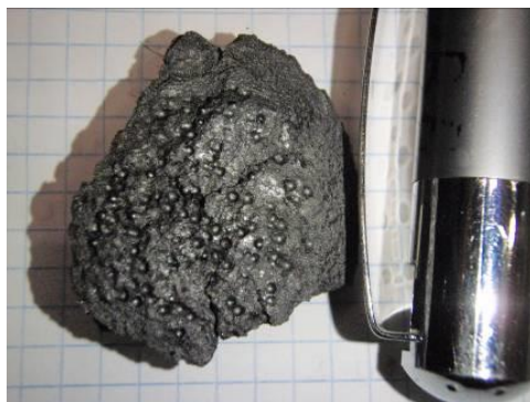
Fig. 6. Crushed fuel pebble after 3 seconds (15 pulses)
