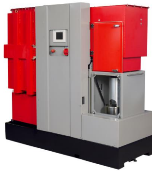
Fig. 5. Commercially available fragmentation machine (“selFrag lab”, height about 2 m)
