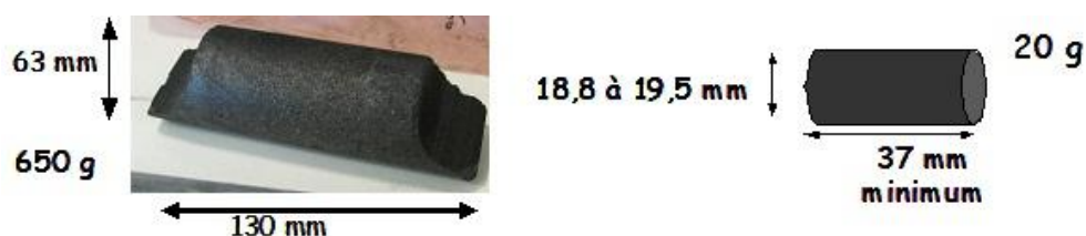
Fig. 12. Graphite samples from CEA G2 reactor (left) and EDF Saint-Laurent A2 reactor (right)
