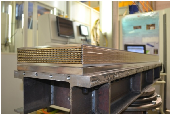
Plate IHX mock-up, manufactured by ALFA-LAVAL and tested in the ARCHER project
