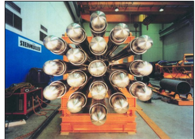
10 MW steam CH 4 reformer mock-up for nuclear application
