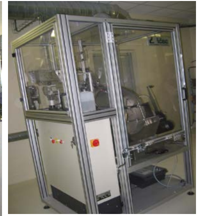
Manufacturing of compacts (CERCA / AREVA)
