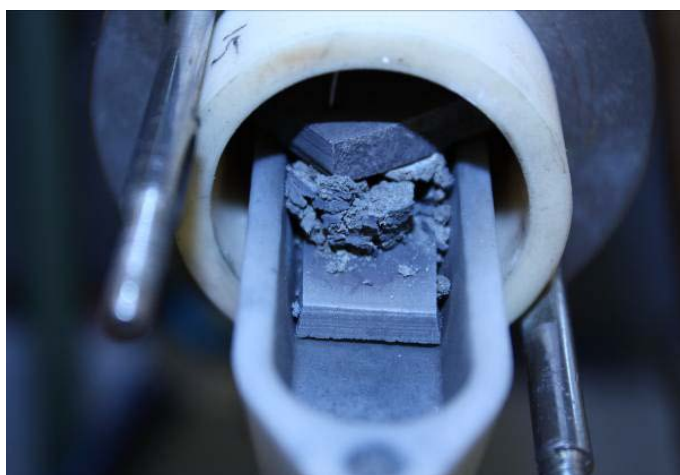
Figure 6.3: A SiC pellet after the Morancais SHS method
