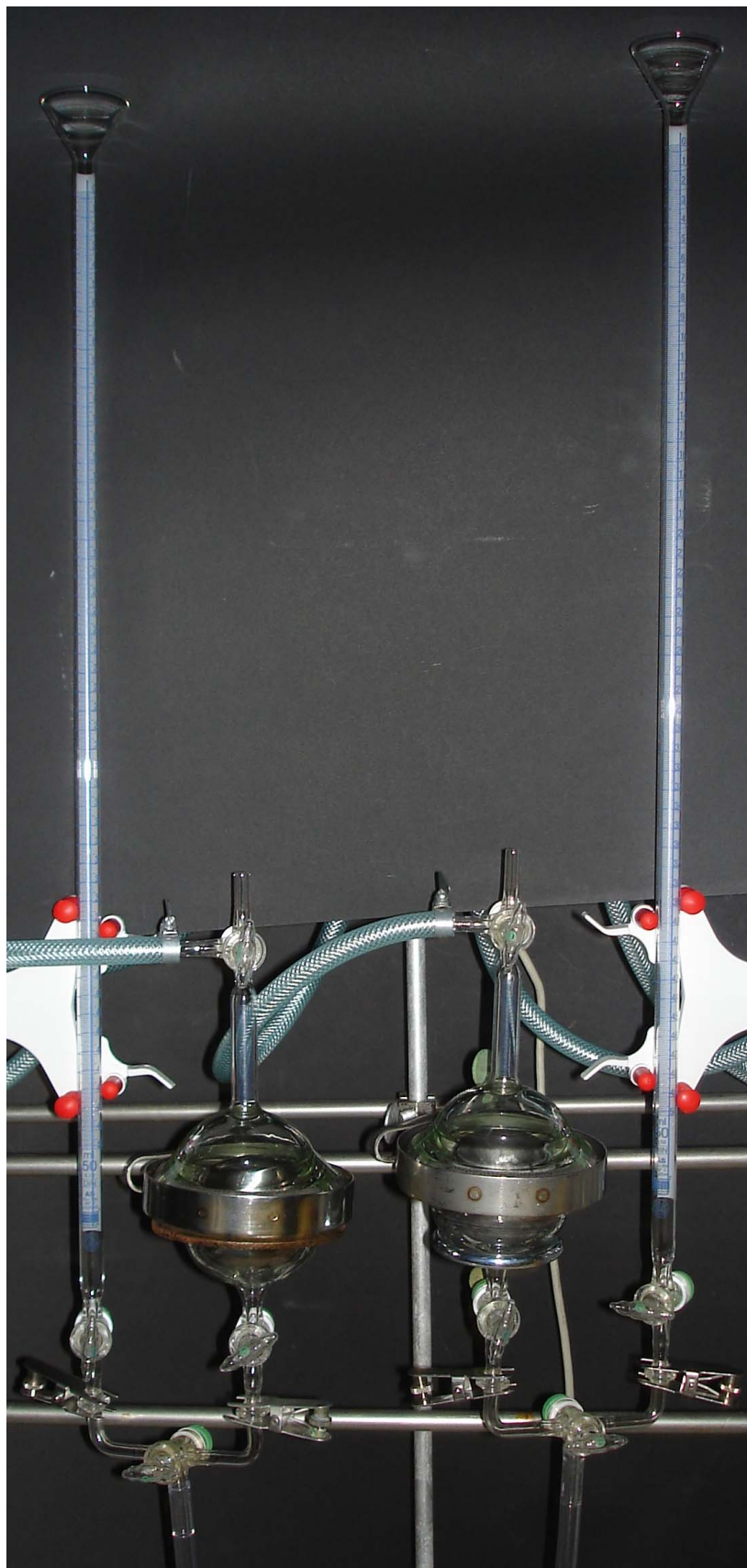
Figure 2: Spherical flasks with graphite pebbles
