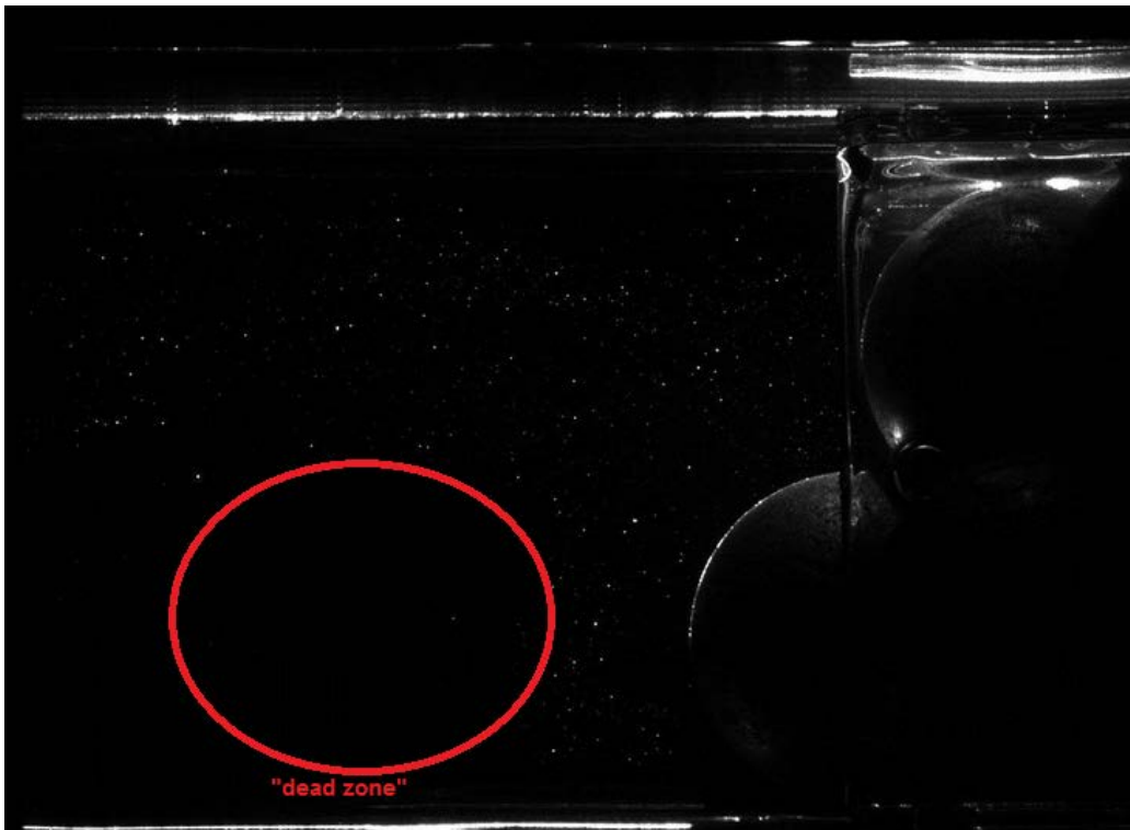
Figure 26: Flow field above the 30mm pebble bed with a "no particle" zone
