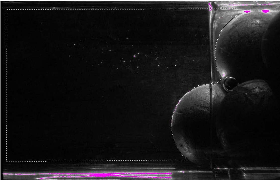
Figure 9: Example of the Mask: the pebbles will be neglected for the Evaluation
