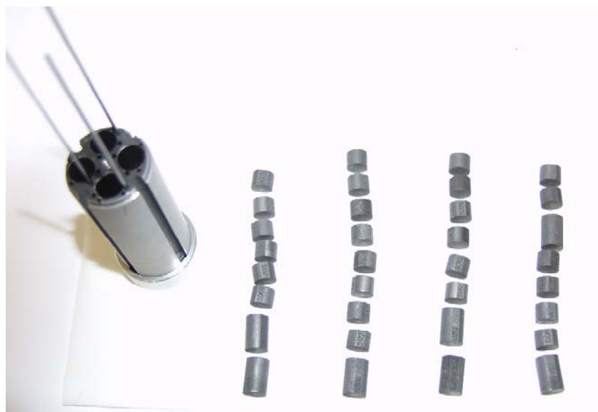
Figure 3 TZM drum and its loading that consists of four columns of graphite specimens (INNOGRAPH-01A).
