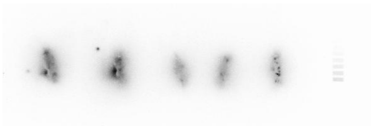
Figure 37 Post treatment 800°C 1%O 2 Autoradiography analysis of samples OM 1, 2, 6, 11 and 13
