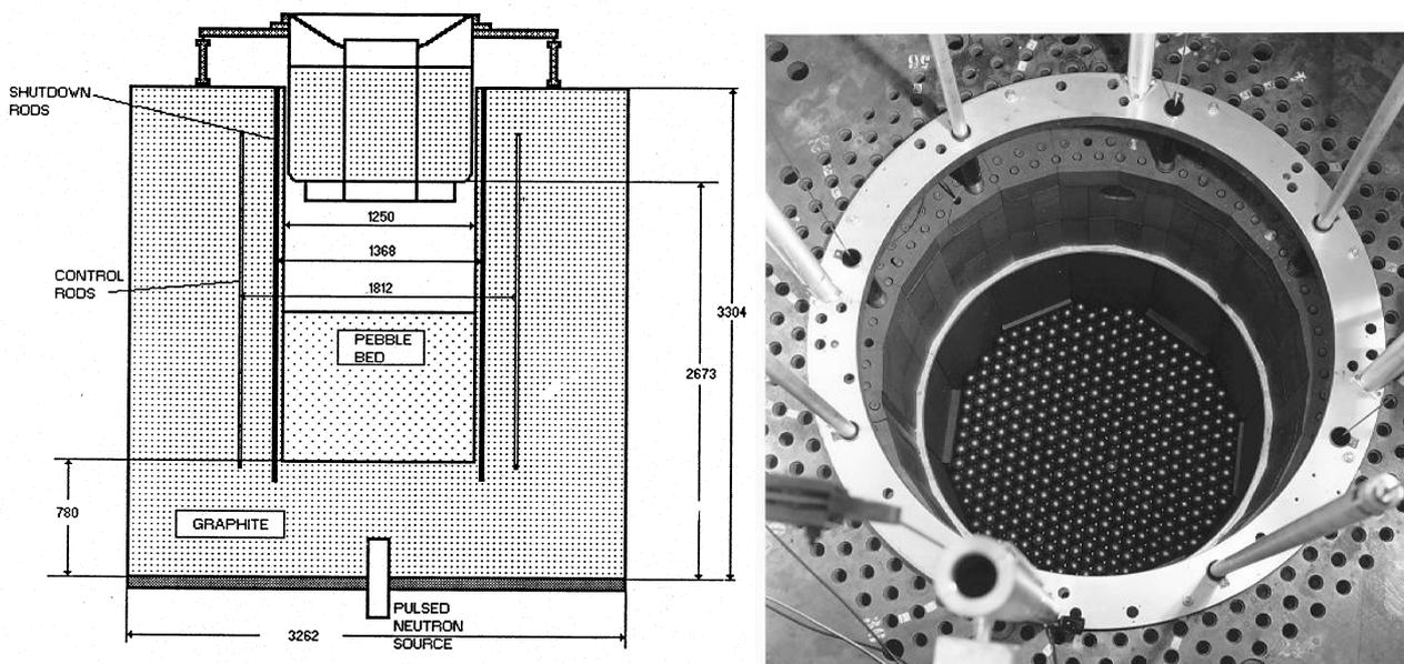
**Fig. 1:** Vertical cross-section of the HTR-PROTEUS-configuration (dimensions in mm, left) and top view of the pebble-bed (right)
