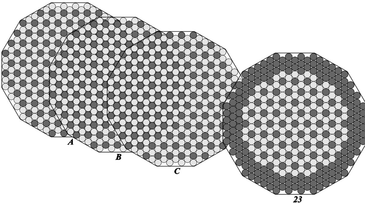
**Fig. 2:** Pebble Layer Structure of HTR-PROTEUS Core 5 with an ABC, ABC... loading scheme. Only the top Layer (Layer 23) was different. Fuel- (grey) and Moderator-Pebbles (black)
