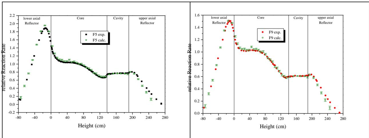
**Fig. 4** Experimental and Calculated (MCNP-4B) axial Reaction Rate Traverses of Fission in  $^{235}\text{U}$  (F5) and  $^{239}\text{Pu}$  (F9) in Core 5.
