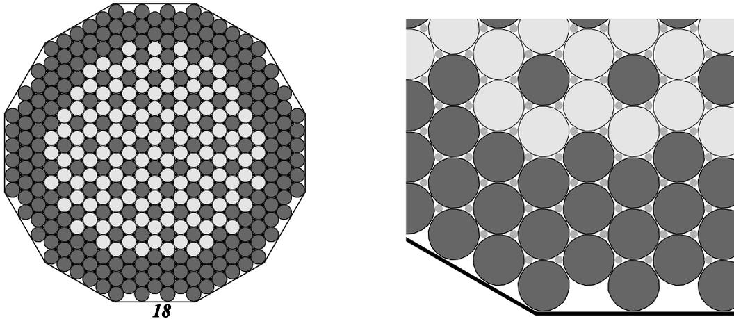
**Fig. 3:** Structure of top Layer 18 of HTR-PROTEUS Core 7 (left) with Fuel- (grey) and Moderator-Pebbles (black). Enlarged area of top Layer (right) with Polyethylene-Rods in the vertical Channels.
