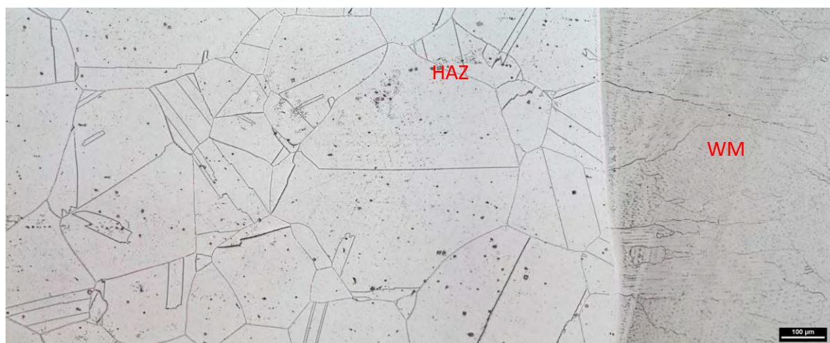
Figure 55: Microstructure of the cross section of the HAZ-WM boundary of the specimen 5S exposed in HTHL during test operation during 665 hours
