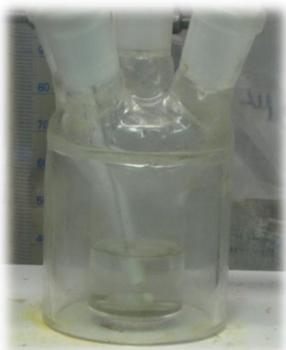
Figure 6 : Picture of dissolution of \text{PuO}_2 sample in \text{HNO}_3 8.5M 95^\circ\text{C} after 6h (left) Dissolution kinetics of \text{PuO}_2 powders in \text{HNO}_3 8.5M – 95^\circ\text{C} . (right)
