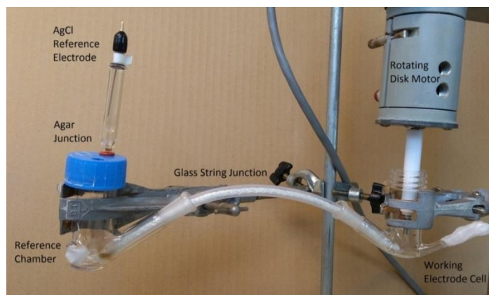
Figure 2: Prototype setup for long term corrosion measurements.
