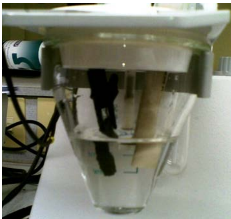
Figure 2.1: Electrolytic cell, where a graphite piece is the working electrode.
