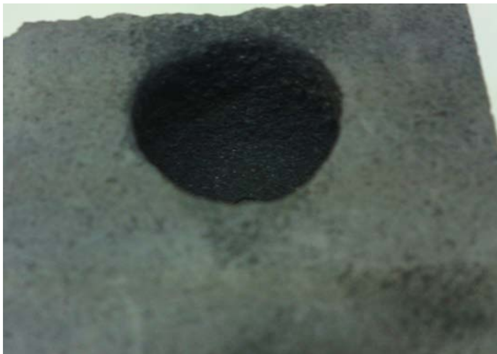
Figure 2.3: Manufacturing of graphite crucibles for molten salt applications using chemical etching technology
