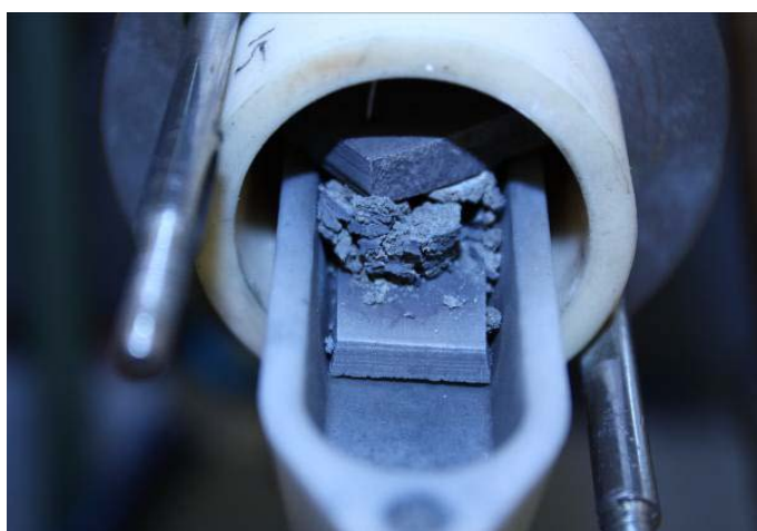
Figure 3.2: A SiC pellet after the Morancais SHS method
