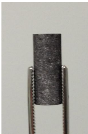
Figure 3.2.5: Small sample used both in the TGA, in the small electric oven and in the Carbolite Oven, H20Ø8 mm
