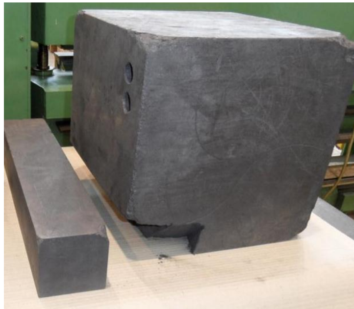
Figure 3.2.3: Coarse virgin material before being cut in smaller samples. Left: Unknown grade graphite, Right: AVR reflector virgin graphite
