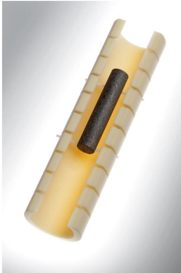
Figure 4.1.7: New sample holder with a virgin untreated graphite sample for the apparatus of graphite thermal treatment
