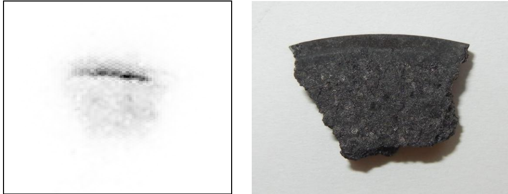
Figure 7.3.2: Spatial distribution of beta-emitters on the surface of the Magnox Oldbury 2 sample from Figure 7.3.1 after thermal treatment determined by digital autoradiography (specimen diameter: 15 mm, thickness: 5 mm, mass: 0.7684 g)
