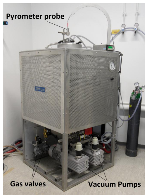
Figure 4.2.5: Overview of the Induction Oven
