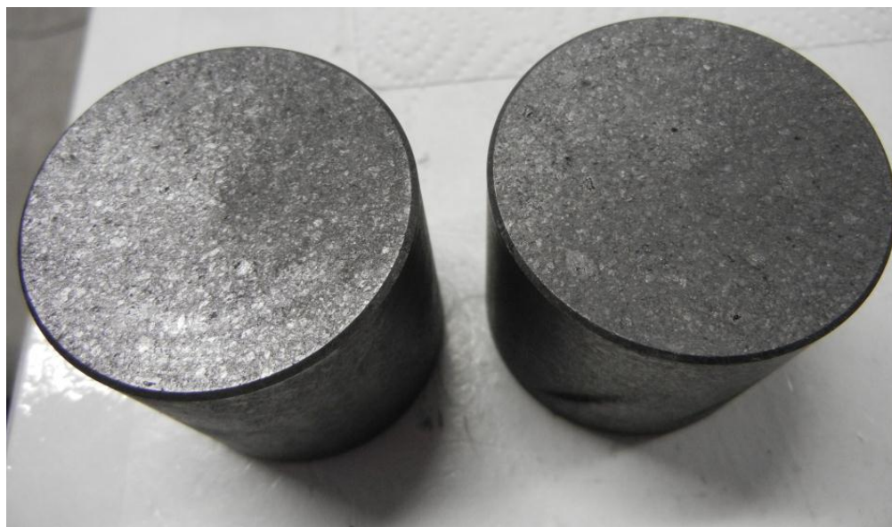
Figure 3.2.4: Massive virgin samples of AVR reflector graphite, H50Ø50 mm
