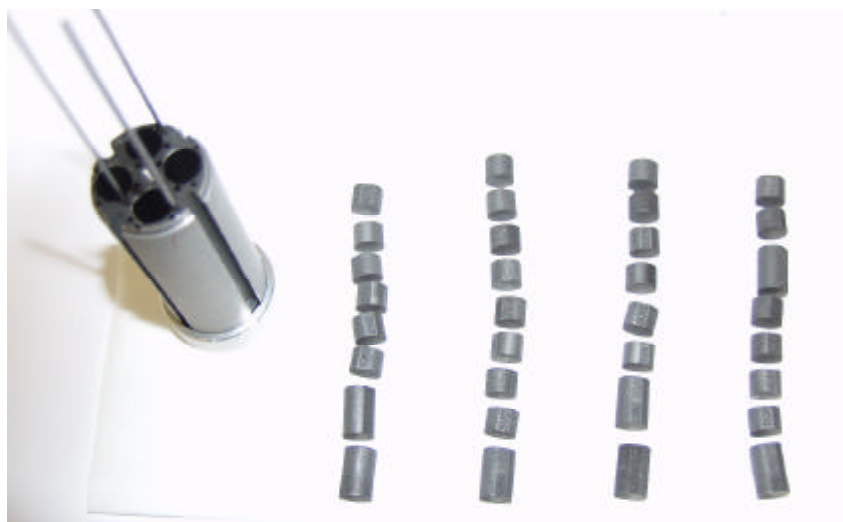
figure 2 TZM drum and its loading that consists of 4 columns of graphite specimens.
