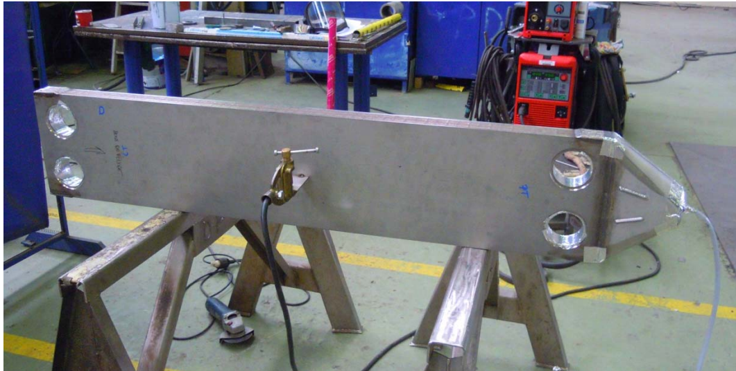
Bundle equipped with its headers (hot circuit)
