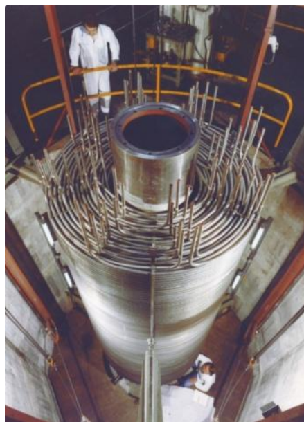
Figure 3-2: Manufacturing of a THTR-300 HX helical tube bundle.
