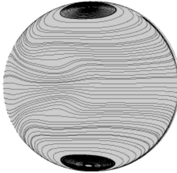
Figure 19 Streamlines of time-averaged flow immediately after the bend.
