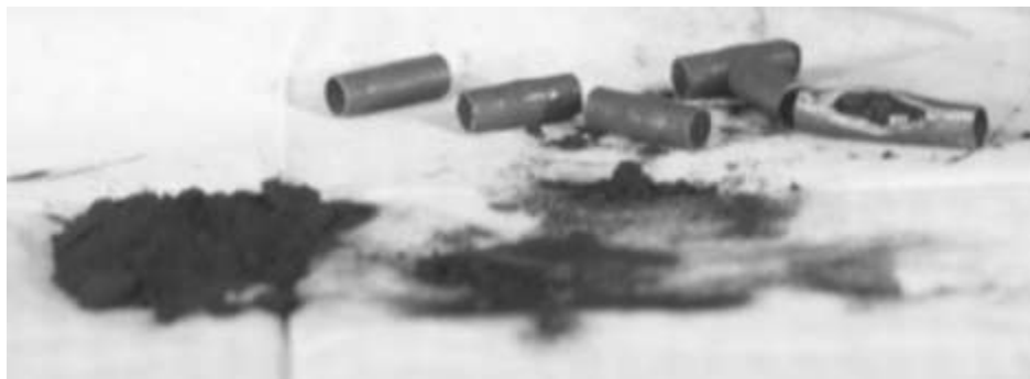
Figure 12 - Spent Nuclear Fuel Post Voloxidation [19]
