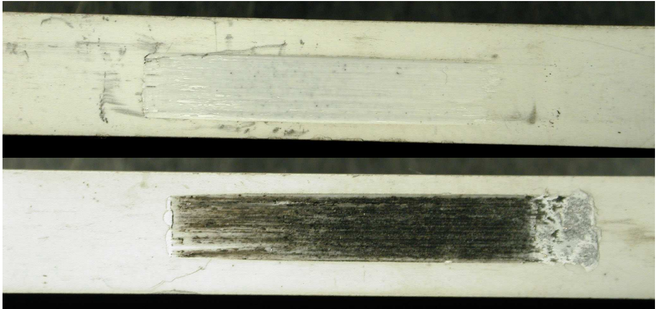
figure 5 : Friction surfaces of the rail coated by Zirconium after 1500 cycles under 800°C and 5 MPa of contact pressure.
