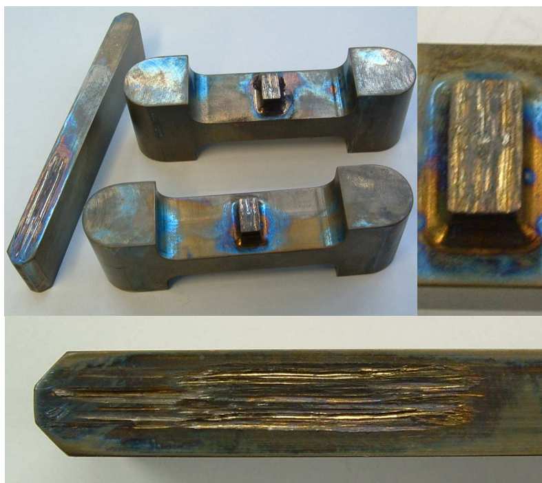
figure 2 : Friction surface of HR230 after 2600 cycles at 450°C under 5 MPa of contact pressure
