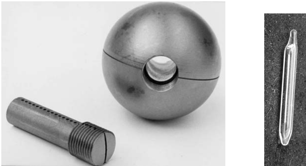
Figure 3. Temperature monitoring sphere prepared for the HTA-8 experiment [Gottaut 1990].
