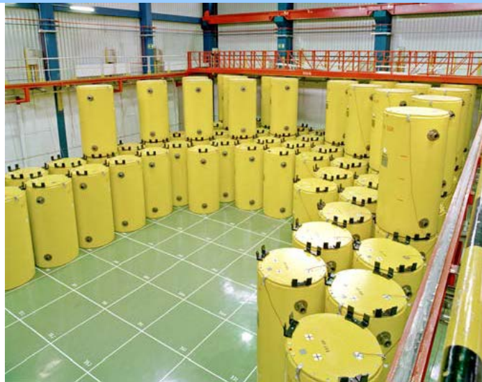
Fig. 6.3: THTR/AVR CASTOR containers stored at Forschungszentrum Jülich, Germany
