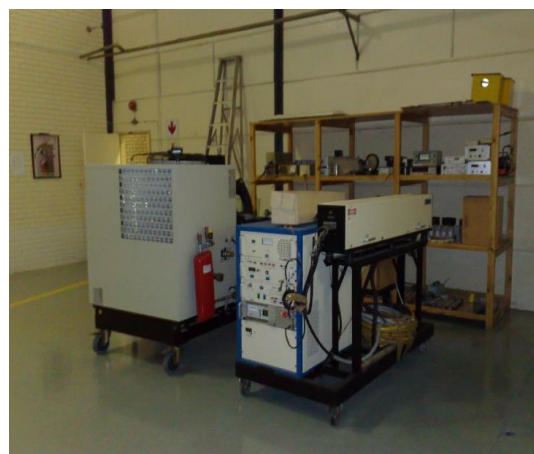
Figure 2. Experimental setup of Nd:YAG laser ablation system at Necsa.
