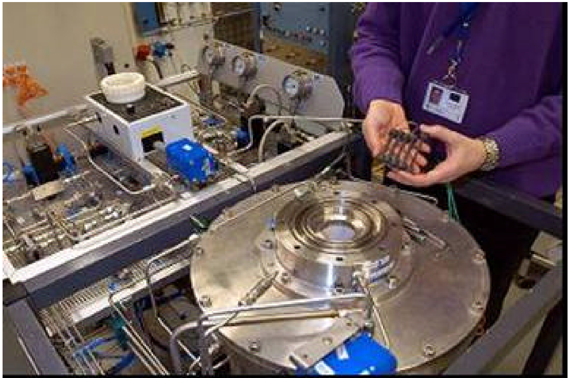
Figure 1 : Carburisation furnace built at JRC.
