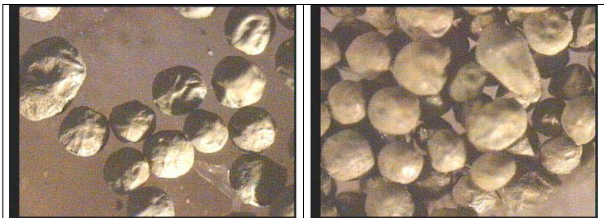
Figure 4.10 : \text{UO}_2 kernels following thermal treatment at 650 °C in Ar/H 2 with normal ageing (left) and ageing with heat treatment (right)
