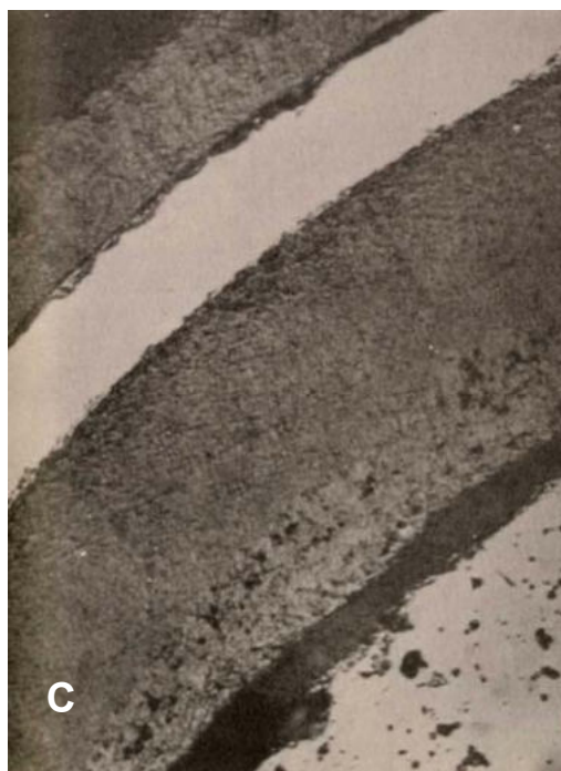
Figure 6: Metallographic cross section of coated particles without overcoating (Batch TN 3/8/2F, 1.45-1.34 %FIMA 1280 \pm 90 °C)
