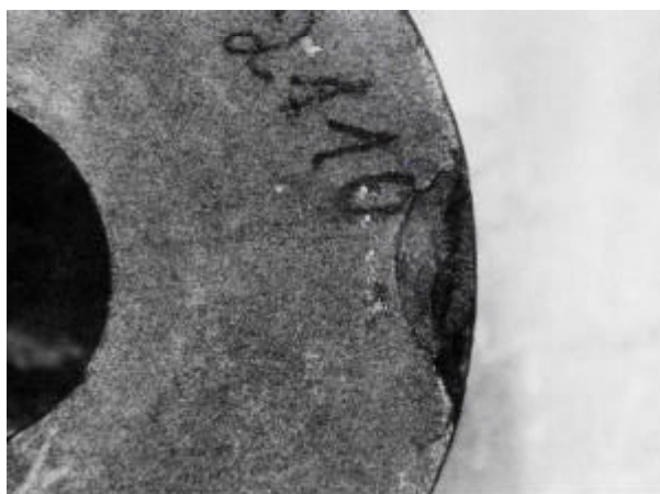
Top end, chipped edge, Compact 2110, position 18
