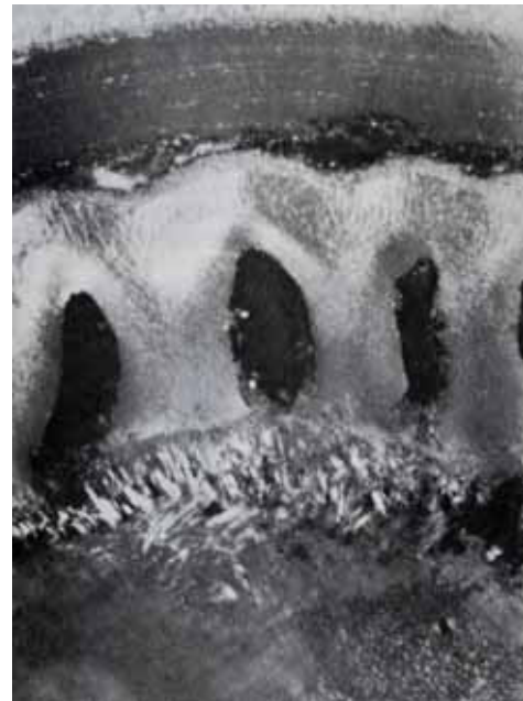
Figure 34: MET V (3) – Metallography of Pu type C particle (Carrier B3-11, tray 8, T=400°C)
