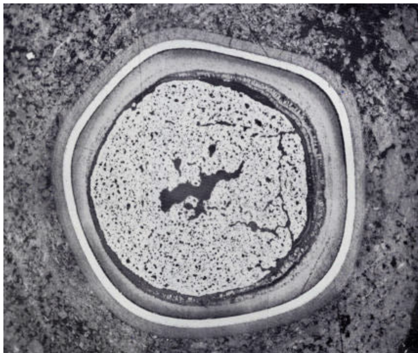
Figure 13: VC02 irradiated compact n°15 - Powder agglomeration coated particle
