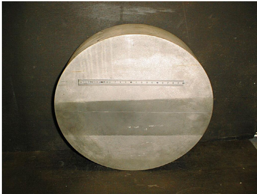
Figure 1 : U720 forged disk used in HTRM project ( \phi=32 cm).
