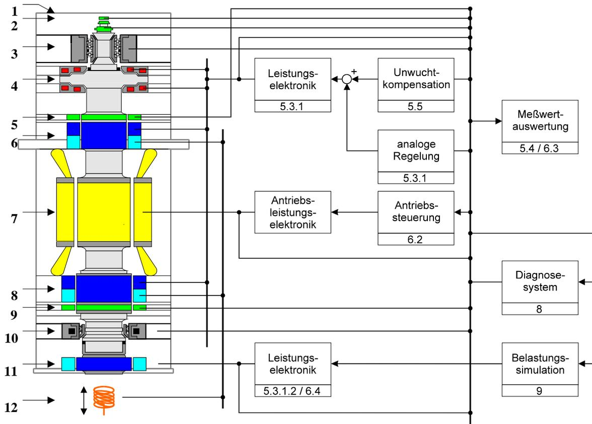
1 ... Test Vessel; 2 ... Axial Sensor; 3 ... Axial-Radial-Catcher Bearing; 4 ... Axial-Magnetic Bearing; 5 ... Top Radial Sensor; 6 ... Top Radial-Magnetic Bearing; 7 ... Asynchronmotor; 8 ... Bottom Radial-Magnetic Bearing; 9 ... Bottom Radial Sensor; 10 ... Radial Catcher Bearing; 11 ... Magnetic Load Simulation; 12 ... Thermal Heating System
