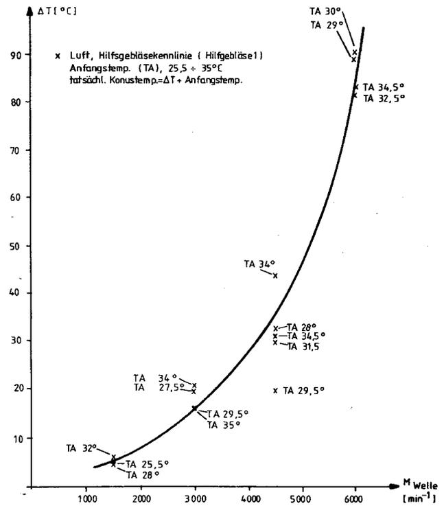
b: Temperature Rise in Friction Cones
