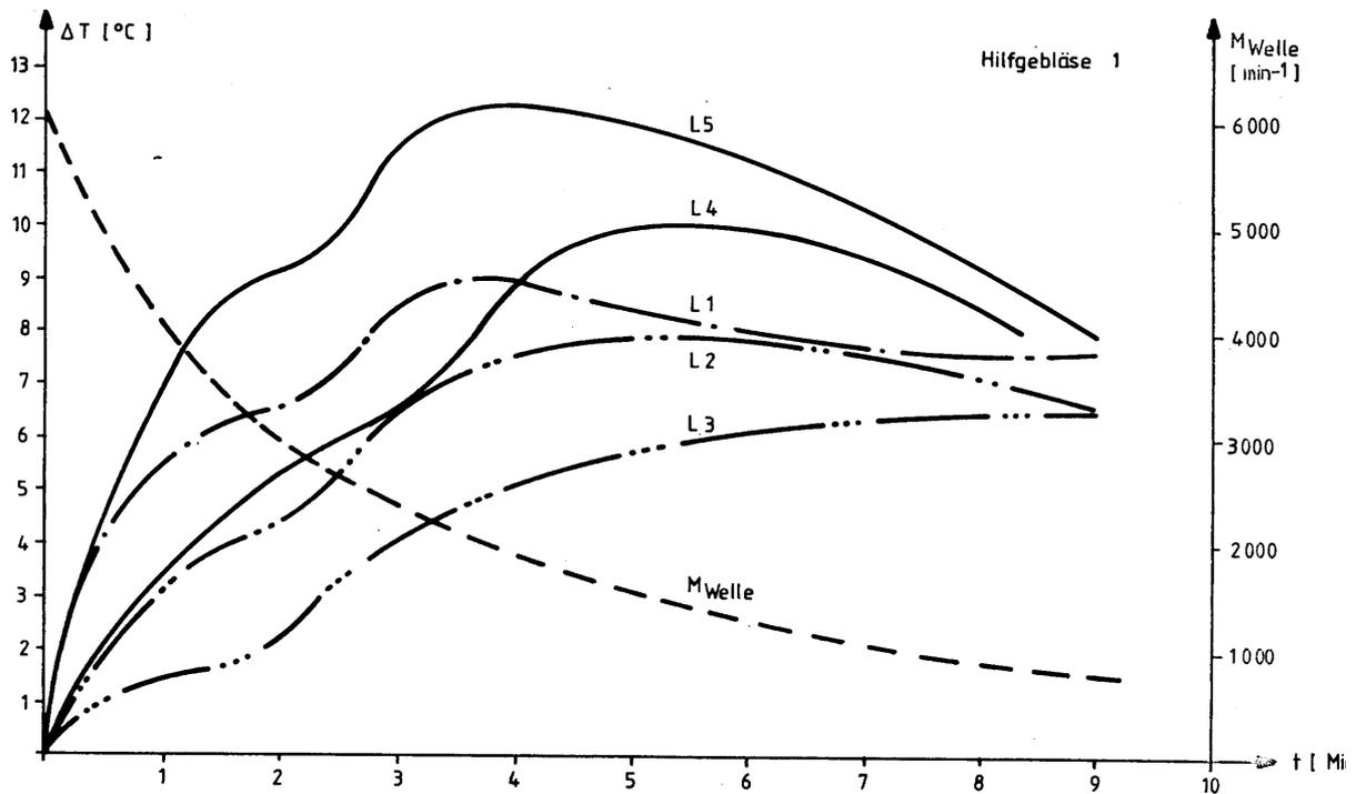
Figure 6.3: Temperature Rise of the Ball Bearing Rings during Coasting of Rotor
