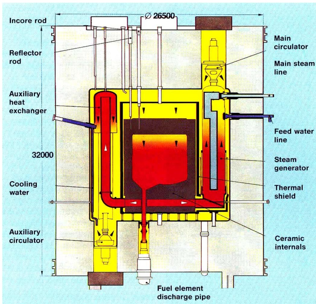
Figure 2.1: Cross-section of HTR 500
