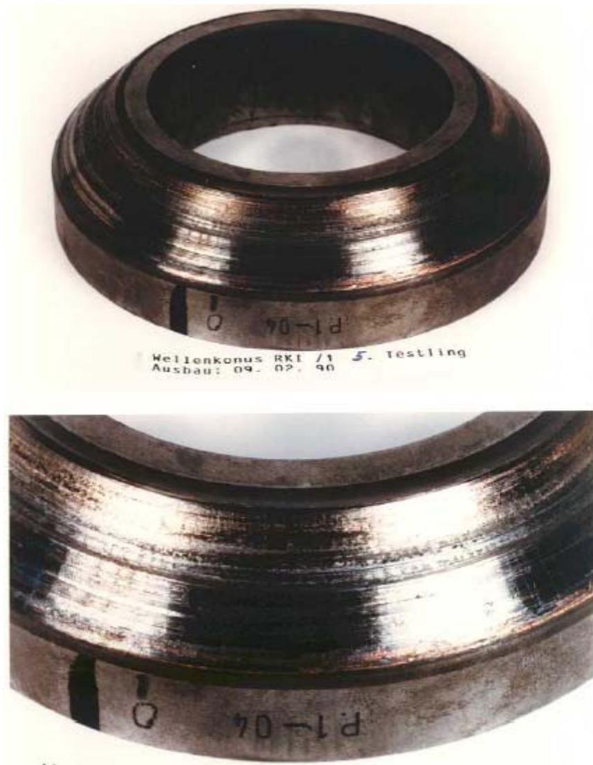
*Figure 6.4: Friction Cone (RK1) after test*
