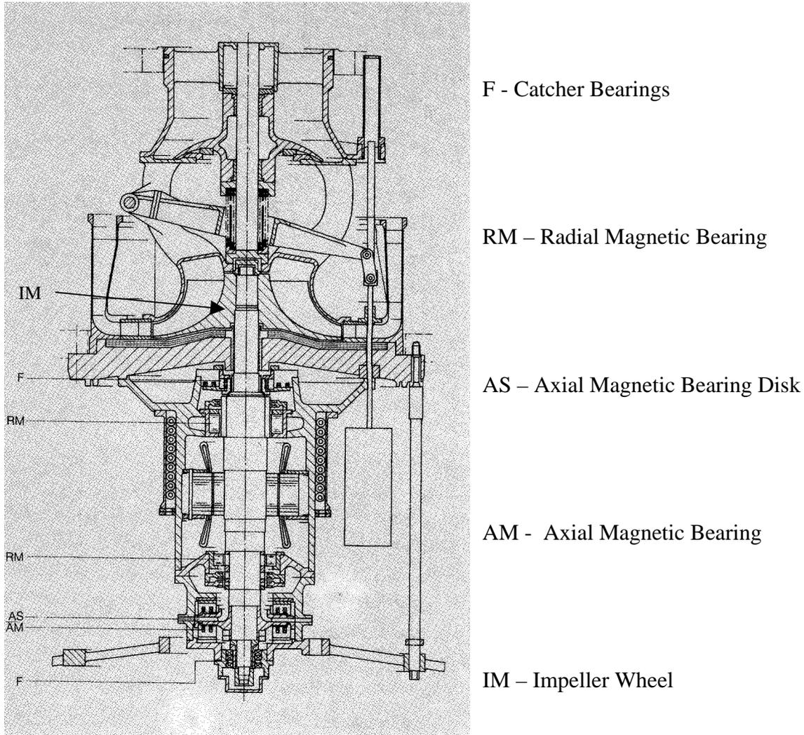
Figure 3.1: Cross section of vertical circulator prototype (MALVE 1)
