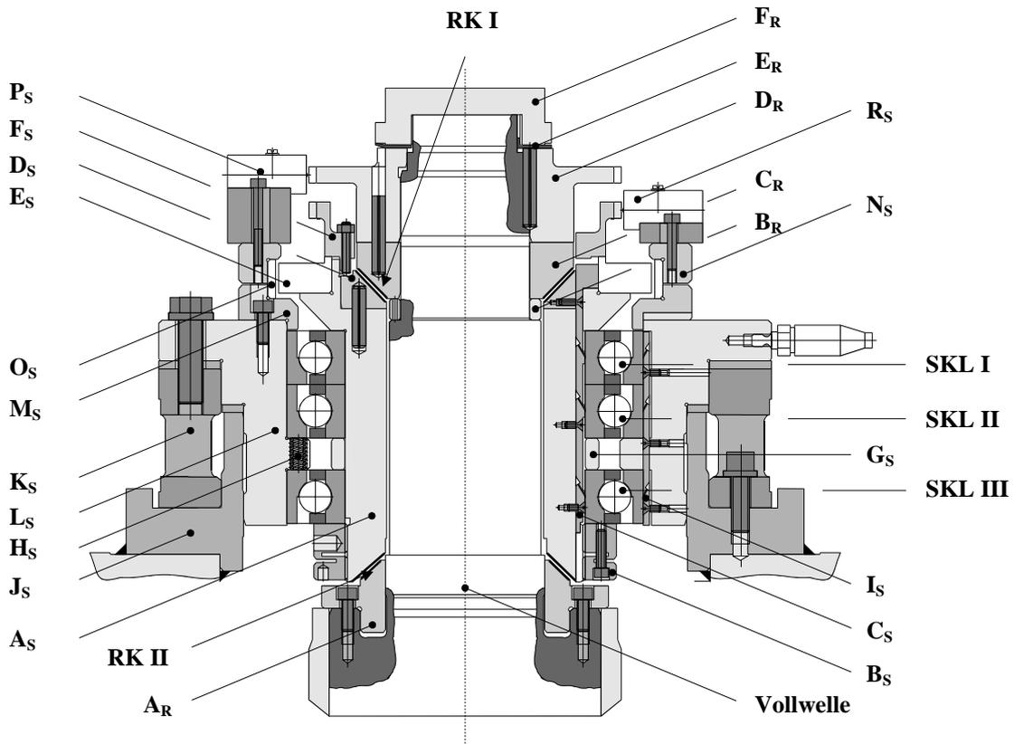
$A_R$  ... Zentrierring,  $B_R$  ... Distanzring,  $C_R$  ... Reibring;  $D_R$  ... Zentrierbüchse,  $E_R$  ... Sicherungsblech,  $F_R$  ... Wellenmutter
