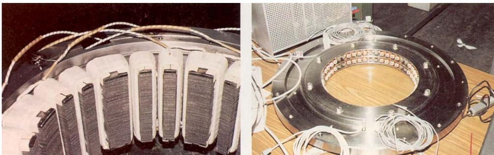
Figure 4.3: Radial Stator of Magnetic Bearing and Sensors (360 mm diameter)
