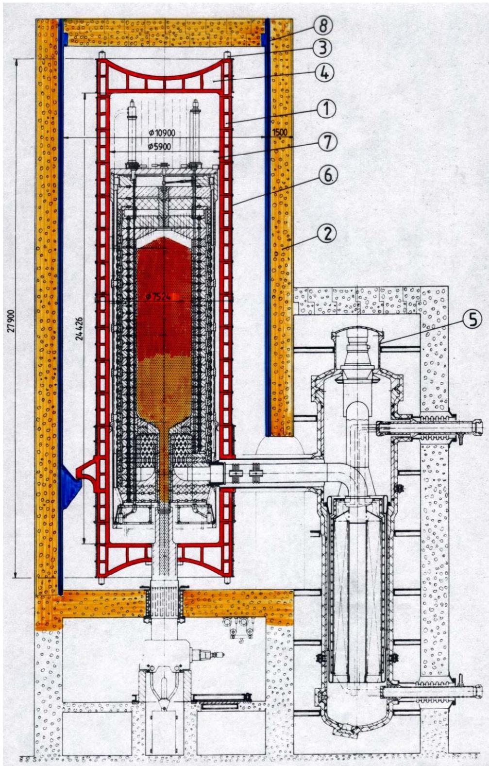
Figure 2.2: Blower (5) position in a HTR Modul (here with pre-stressed cast-iron vessel)
