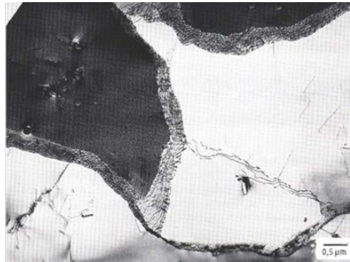
Figure 2-21: Subgrain boundaries in Alloy 800H after creep load [33]
