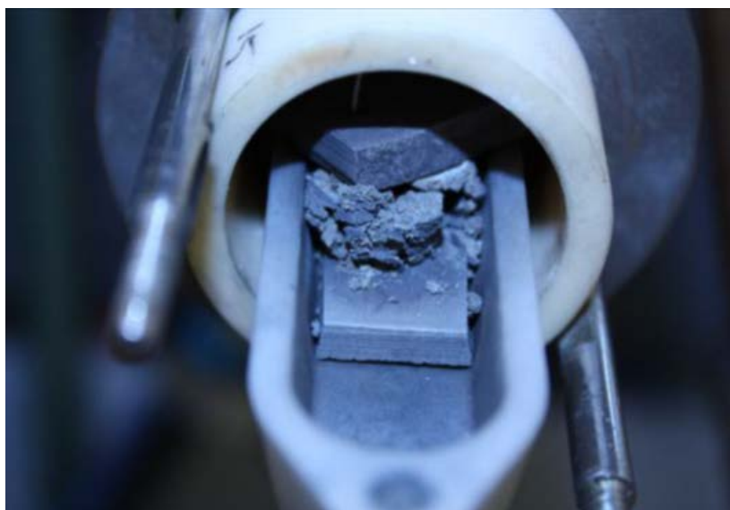
Figure 5.2: A SiC pellet after the Morancais SHS method
