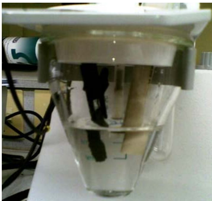
Figure 7.1: Electrolytic cell, where a graphite piece is the working electrode.
