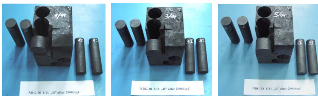
Figure 3.3: Samples after graphitization (from left to right: Reference, Trial 1 with 7.5 % carbon black, Trial 2 with 15 % of carbon black), with core samples already taken
