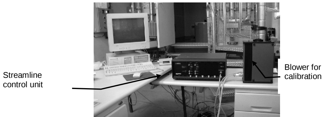
Figure 3 – The high frequency hot wire anemometry system (Dantec)
