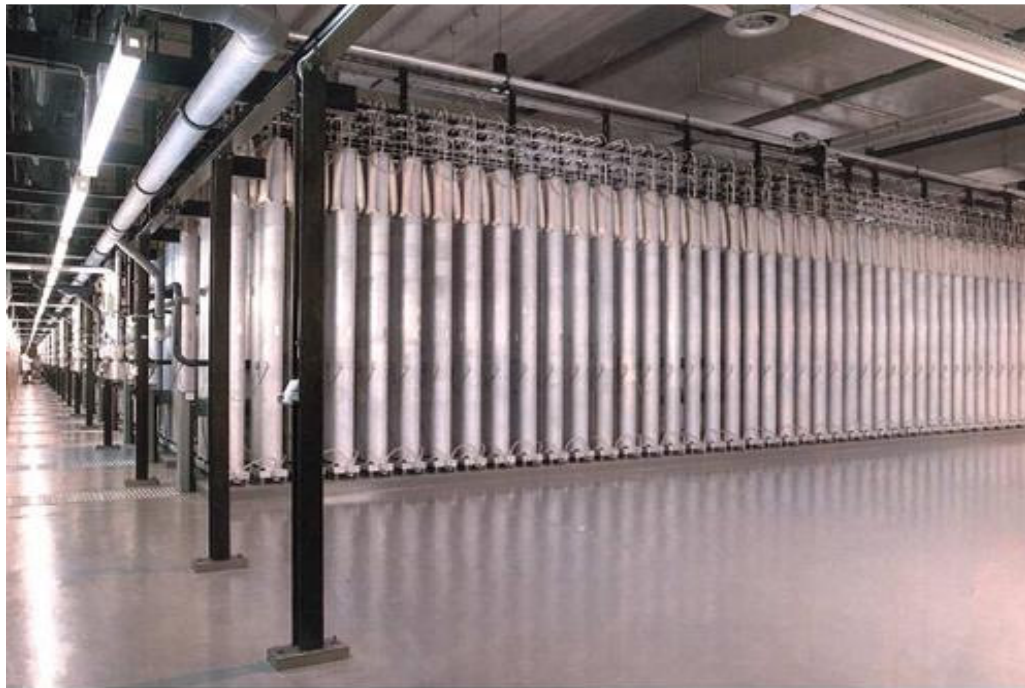
Figure 3.5 - A cascade of gas centrifuges at a URENCO plant.
