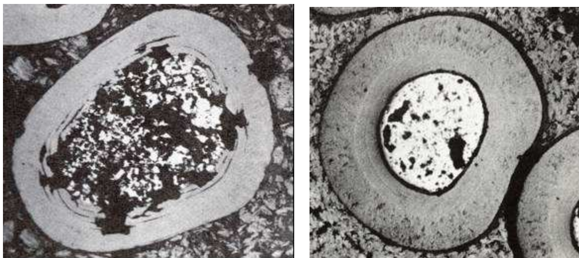
Figure 68 : Irradiation results on (Zr,U)C coated particle fuel [Price 1966]
