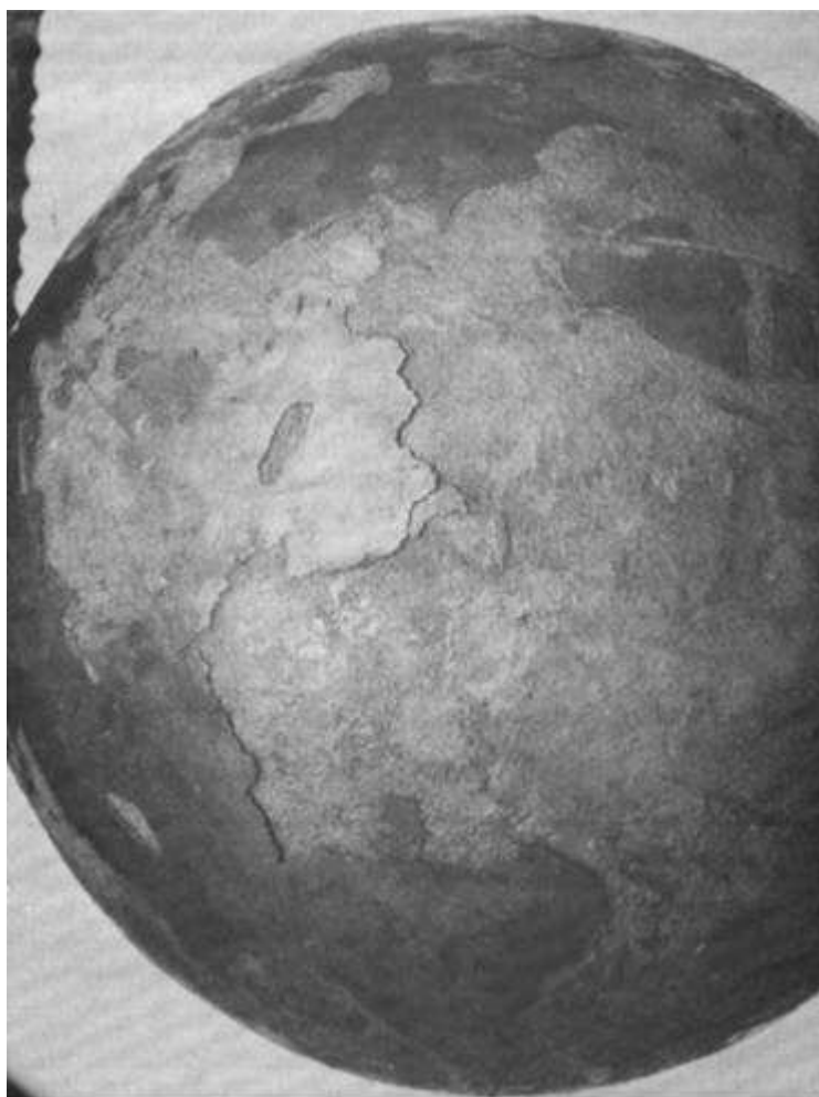
Figure 48 : Peeling effect observed on AVR fuel sphere surfaces [Burck 1977]
