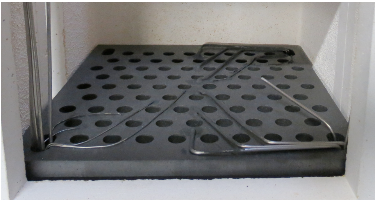
Figure 12: Example assembly of thermo couples in an experimental set up for fluid dynamics investigation done in NACOK II previously
