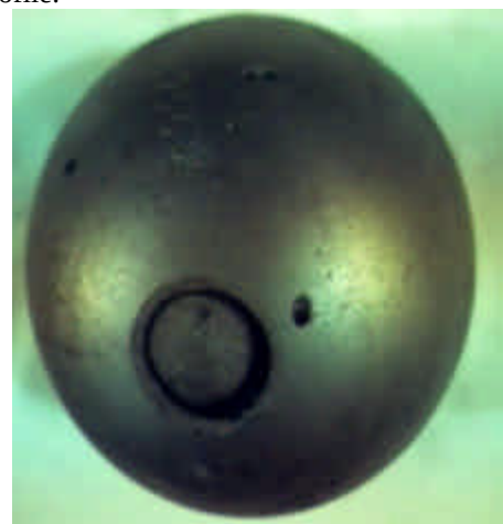
Figure 8: Carottage of an irradiated pebble after KÜFA-test
