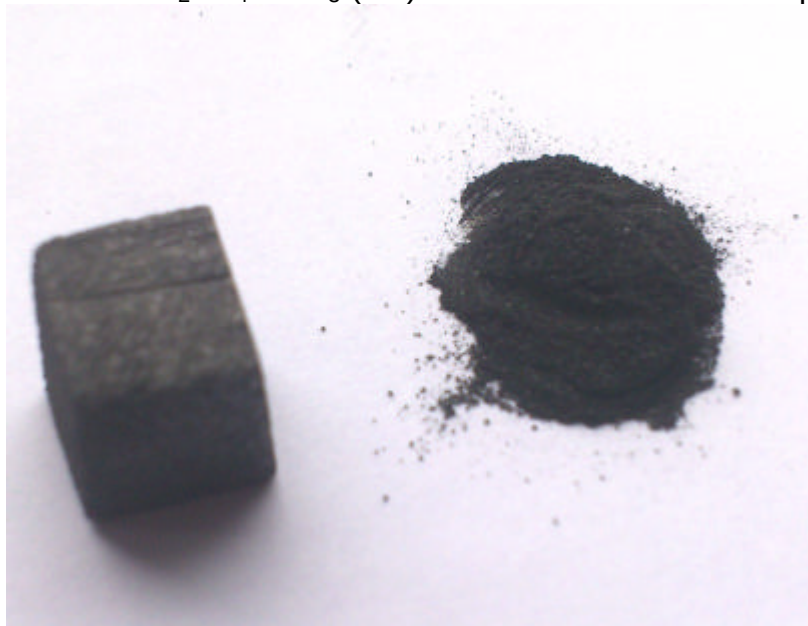
Figure 31 Virgin graphite block and graphite powder obtained after the treatment with the mixture \text{H}_2\text{SO}_4:\text{HNO}_3 (4:1)
