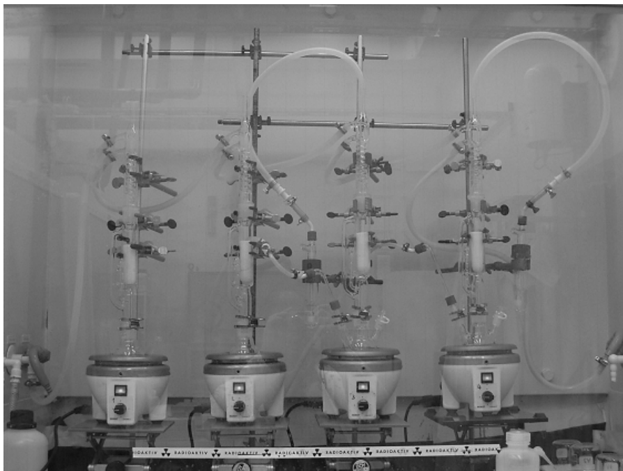
Figure 5: Experimental set-up for the Soxhlet extraction for the Merlin graphite
